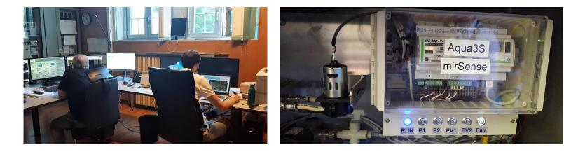
Anomaly detection based on almost real time data acquisition from monitoring sensors and numeric simulation models. The system allow associating to qualitative and quantitative variables a set of threshold values, defined by user as representative of an anomaly situation (i.e. drought, a flood, a contamination etc.). In case of data acquisition out of the range, automatic warning is provided. Possible operational scenario are also available according to the specific anomaly event triggered
